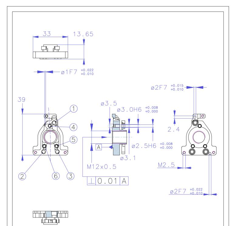
Note: protect cylindric surfaces 1, 2, 3, 4, 5 and 6 from anodizing.
